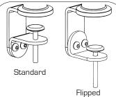
\*The C-Clamp will accomodate thicker surfases if the C-Clamp Bottom Bracket is flipped
