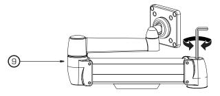
Position Arm so it is parallel to desk surface. Turn bolt clock wise for lighter monitors.
