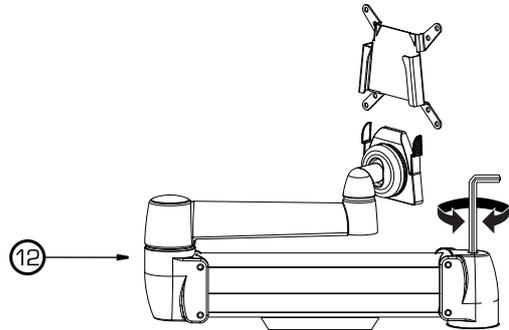
Position Arm so it is parallel to desk surface. Turn bolt clock wise for lighter monitors.
